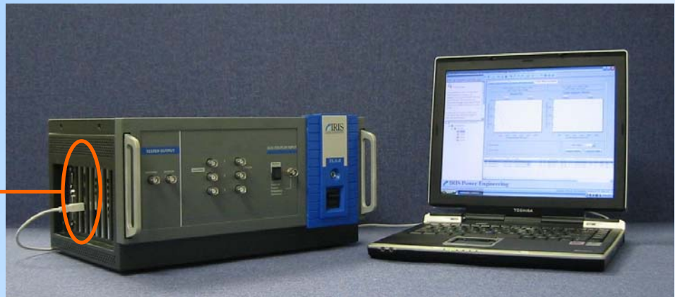
PDA-IV instrument with low frequency option. The laptop controls measurement process and stores test results
