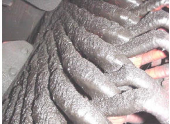
Figure 7. Detected contamination of end-winding with oil and dust.
