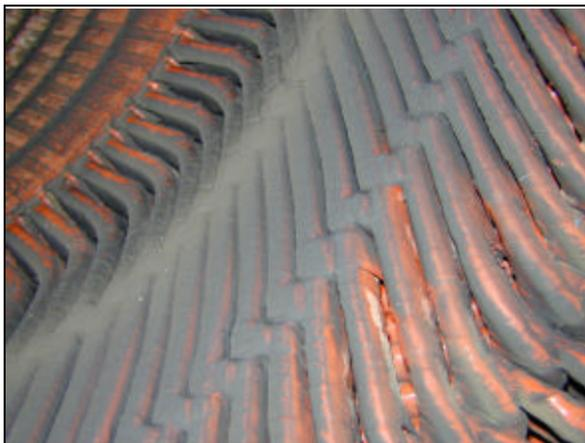
Figure 6. Detected surface contamination. Example of reversible problems detected in a 6.6kV Epoxy-mica insulation machine.
